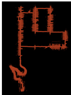
(j) LiDAR map of mine environment (rock walls and tunnels)
